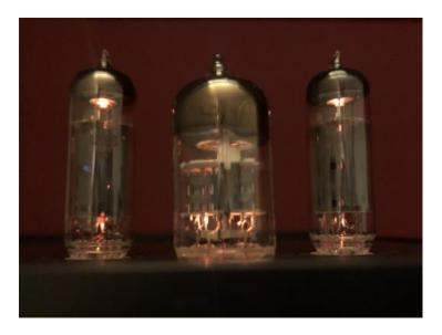
Within about 20-30 seconds from switch on the amplifier will be starting to work (it can take up to 5 minutes to reach full specification).
